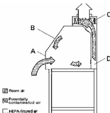
Class I cabinets offer good protection for the operator and the environment, and are simple and economical to operate. Radioisotopes and some toxic chemicals can be used (if the cabinet is ducted to the outside), but HEPA filtered air is not provided over the work area. Thus, these cabinets do not protect your materials from contaminants introduced from the environment or the operator.
