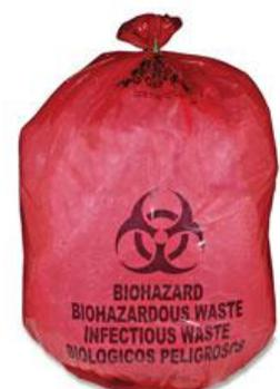
with biohazardous materials into red bags that have the biohazard symbol or the word "BIOHAZARD". Use double bags if necessary to prevent leakage.
