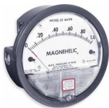
Observe the magnehelic gauge and note its relative position each time you operate the BSC (e.g., maintain a log). The magnehelic gauge measures the pressure drop across the HEPA filters, and thus indicates filter load and integrity. An increase or decrease in the pressure value may indicate clogging or leaking of the filter, respectively.
