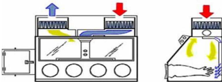
Class III cabinets provide maximum protection to the environment, the worker, and the product, and are used with high-risk agents. These cabinets are gas-tight enclosures and the interior is accessed through a dunk tank or a double-door pass through box. Supply and exhaust air are HEPA-filtered
